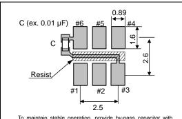
To maintain stable operation, provide by-pass capacitor with more than 0.1  $\mu$ F at a location as near as possible to the power source terminal of the crystal products (between Vcc - GND).
